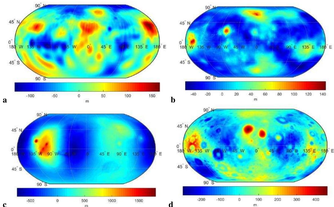
Figure 8: Geoidal heights on (a) Mercury, (b) Venus, (c) Mars and (d) Earth's Moon.
